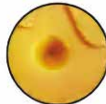
Test Results at 59°F Hammer Dropped at 12.5ft
