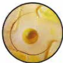
Test Results at -43.6°F Hammer Dropped at 8.5ft
