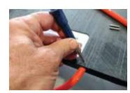
Position the pad off the edge of a table or sturdy work surface so the pins will clear the table when coming out of the backside of the pad.
