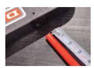
Turn the pad over and insert the ends of the new handle into the holes. Make sure the ends are seated in the holes, with a minimum of 1" of handle into the hole.
