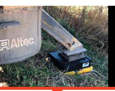
DICA's ProStack Slot Lock Blocks can stack and interlock for optimum stability, giving operators the safety and versatility they need when working in unlevel conditions. The patented design integrates with SafetyTech Outrigger Pads to increase bearing area. Slot Lock Blocks are designed for both operating equipment and static load applications.
