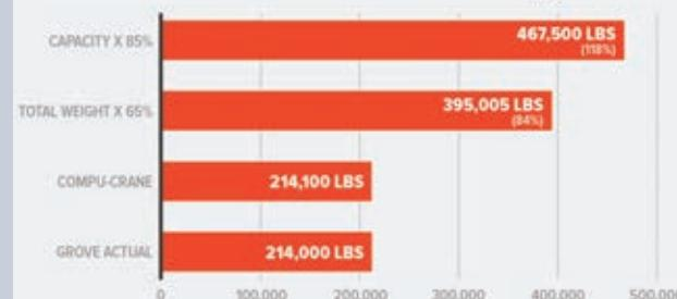
In this example, the two rules of thumb overestimate MORF by 118 percent and 84 percent. In contrast, the Compu-Crane software and the manufacturer data provide consistent, accurate MORF information.
