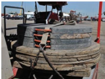
**LEFT: Engineered outrigger pads (top of photo) provide consistent, reliable strength and rigidly properties and are not susceptible to the elements. This is a clear distinction from more commonly used wood outrigger pads whose strength and stiffness properties can be ever changing (bottom of photo).**
