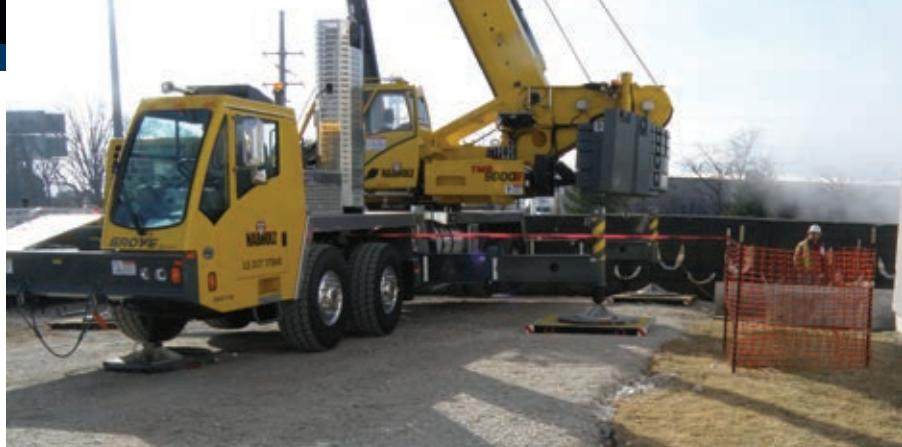
**Nabholz Construction, Rogers, Ark., uses SafetyTech and FiberMax crane pads on top of improved ground that is firm, drained and graded.**
