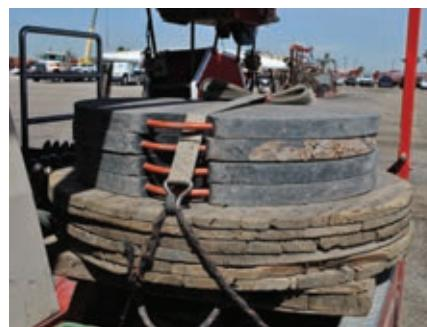
**LEFT:** Engineered outrigger pads (top of photo) provide consistent, reliable strength and rigidly properties and are not susceptible to the elements. This is a clear distinction from more commonly used wood outrigger pads whose strength and stiffness properties can be ever changing (bottom of photo).
